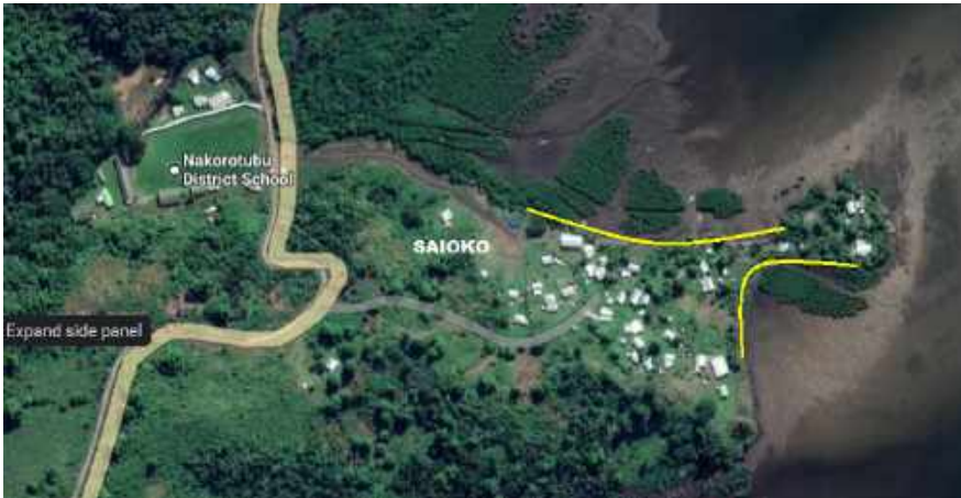
Figure 43 Proposed extent of seawall for Saioko Village.
